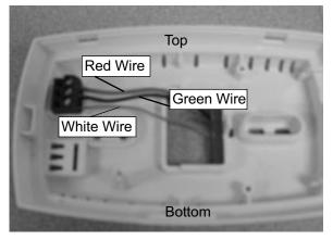
Figure 21.1 - Back Side of Wall Control with Cover Off
